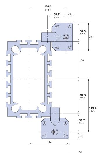
The drawings on this page illustrate various important dimensions when using HDS2 bearing blocks. Additional dimensions can be determined by working from the bearing block dimensions shown in this datasheet as well as component dimensions shown in the full HDS2 catalogue.
