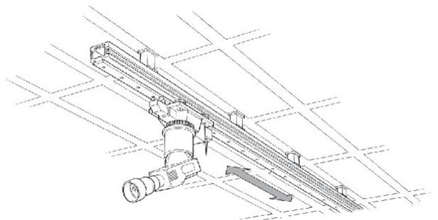
**c)** Incorporating the rack directly to the slide saves on setting a separate component (as described in point 3)
