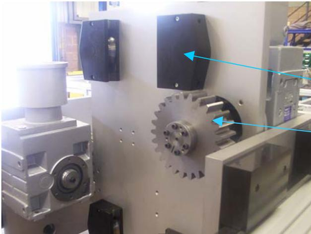
Carriage fitted with low maintenance cap seals with pinion drive in position.
