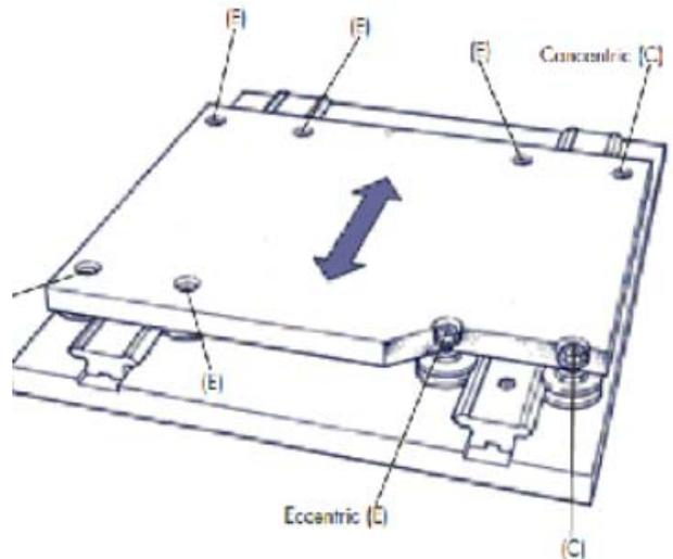
Picture shows the two slides located into two machined slots. Alternatively to achieve sufficient parallelism the slides can be fitted to a clear surface using the dowel pins located into the slide base keyway as stated point 10a
