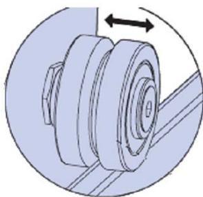
Axial float from floating needle bearing offers compliance
